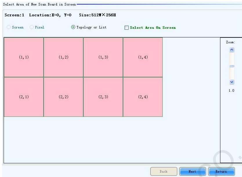
Figure 5-46 The page for specifying the working area of the new receiving card
