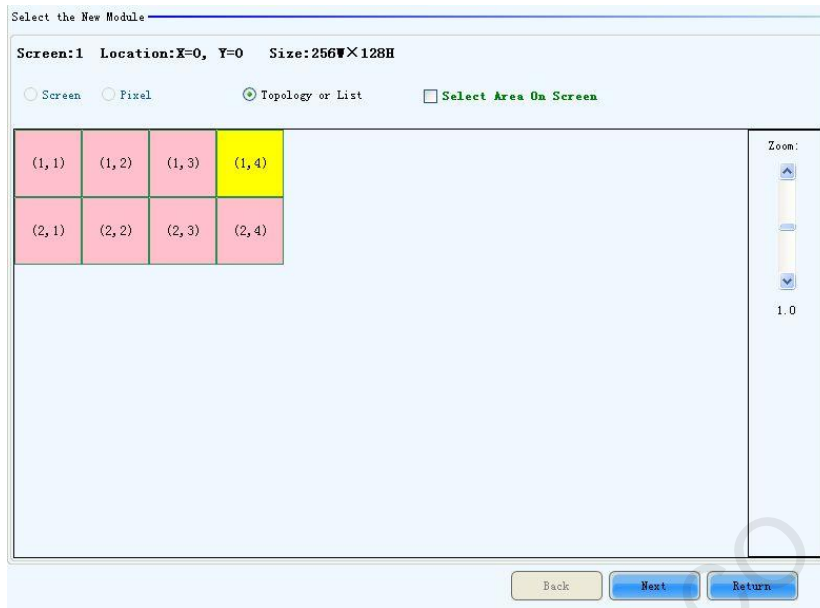
Figure 5-52 The page for specifying the cabinet which the new module is in
